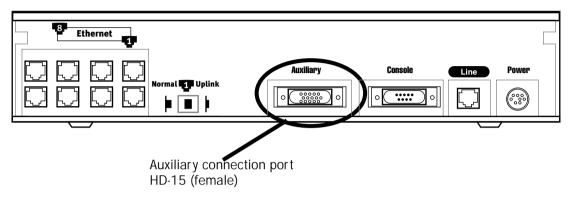
Connect the male HD-15 end of the PhoneNET connector to the Auxiliary port on your Netopia R5000 Series. Connect the other end of the cable to your LocalTalk network. You can use only one connection on the Auxiliary port. You cannot use both the PhoneNET connector and an external modem.
